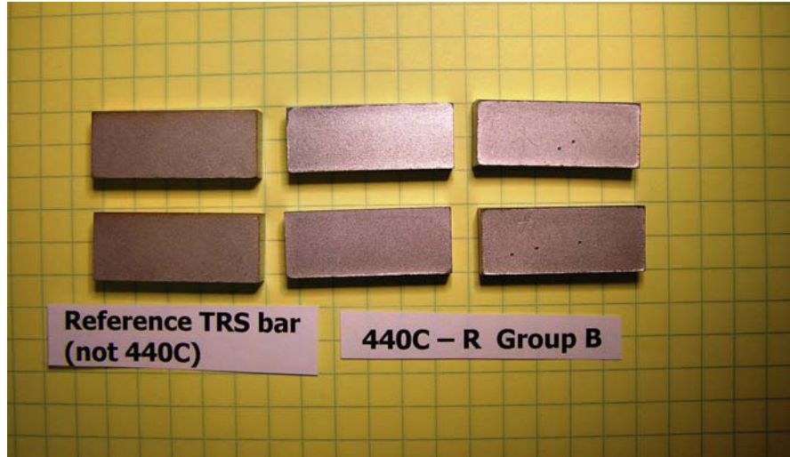
Figure 4: Images of 440C TRS bars (right four) showing the amount of distortion that occurred during liquid phase sintering. TRS bars (two) on the left side were produced from a stainless steel powder by conventional solid state sintering.
