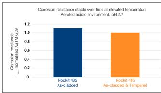
Rockit 485 was tempered at 500°C for 24h in air. The temperature was selected to represent the surface conditions of the caster rolls at steady state.
