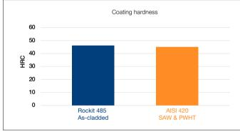
Rockit 485 laser cladded vs. AISI 420 martensitic stainless steel, submerged arc welded (SAW) and post welding heat treated (PWHT).
