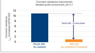
Rockit 485 laser cladded vs. AISI 420 martensitic stainless steel, laser cladded and tempered (500°C, 24h, in air).
