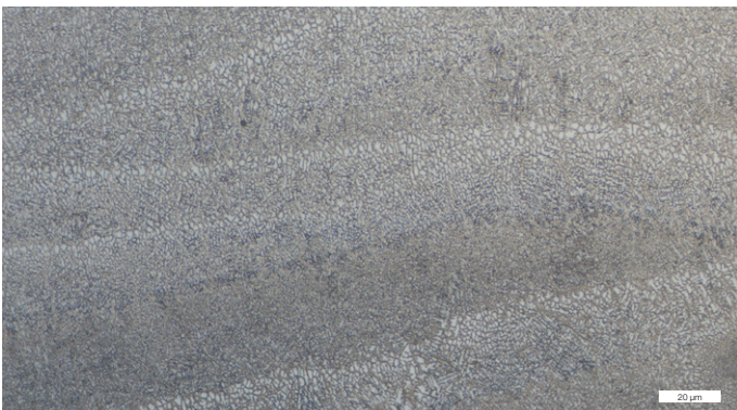
Very fine and homogeneous microstructure consisting of ferrite, martensite and eutectic structure
